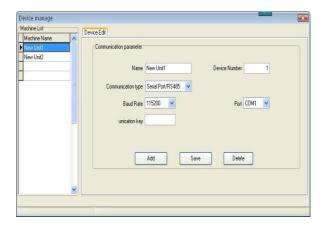
There are two default communication mode provided in the system, one is RS232/RS485, another is Ethernet. Some specify machine is designed with USB communication mode (such as H2), for more detail, please refer to corresponding "User Manual", the using method please view the explanation below:
