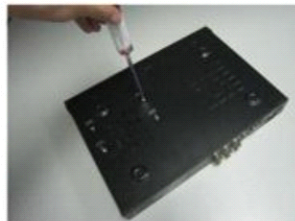
⑤ Fasten the hdd on the Back panel
