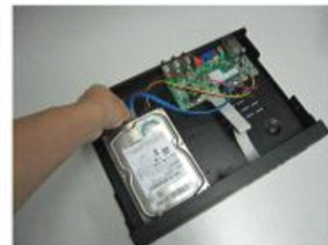
⑥ Insert the power cable On the hdd
