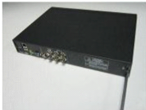
① Remove 2 screws of the back panel
