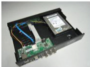
④ Fasten the 4 screws into the slot
